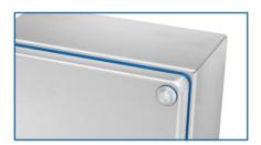
Customized convex blind nut with under head special design for anti-loss purpose equipped with gasket. Threaded path length foreseen for guarantee a certain mechanical stop, to avoid excessive gasket compression.
